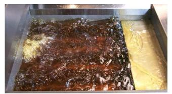
Allow the oil to bubble for 15-30 seconds to ensure evacuation of all oil in the return lines.
